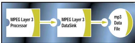
FIGURE 6 Connecting an MPEG DataSink to an MPEG capture device results in an MPEG file being saved.
