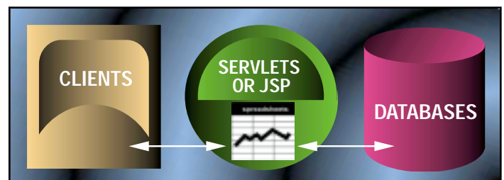
FIGURE 1 Spreadsheets provide an effective means for building business logic in three-tier architectures.
