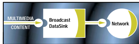
FIGURE 7 A broadcast DataSink can output multimedia content to the Internet rather than a file.
